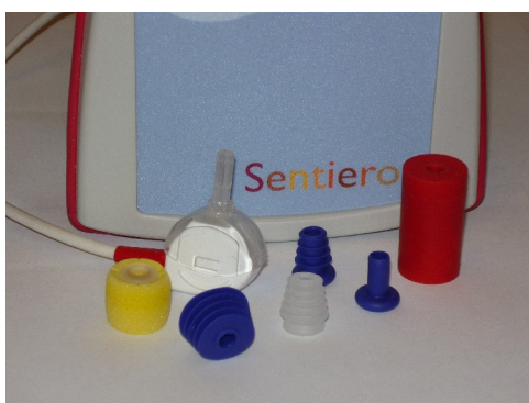
Fig. 24: Test coupler (right), probe with mounted probe tip, ear tips (accessories)
